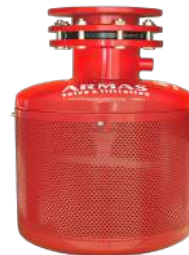
Autoflushing Foot valve with 500micron screen 6"-8"-10"-12" 180-315-495-710 m3/h
