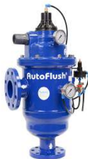
Automatic Screen Filter Hydraulic / Electric 2"-3"-4" 25-50-100 m3/h 15-20-22 m3/h for flushing 16 sec
